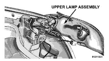
4. Replace the backup or rear turn signal lamp bulb. Reinstall the appropriate bulb and socket assembly. Reinstall the three bulb and socket assemblies in the upper lamp assembly. Reinstall the upper lamp assembly. Replace the access panel. Close the trunk.
